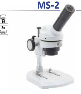
Entry-level monoscope with fixed objective (2x) that can be combined to external illuminators, in case some light is required.
